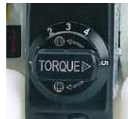
Torque selector With 5 positions
