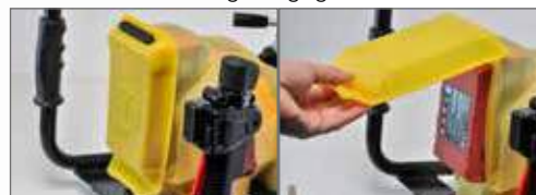
Rainproof cover with opening to change the battery
