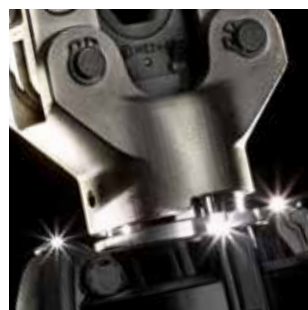
4 LED lighting of the working area
