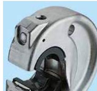
Die release system, protected from accidental operation
