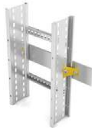
Safe working load 215kg per pair of adaptable fixing brackets when supporting Speedway cable ladder installed as part of a vertical run
