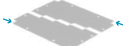
Integral Joint Strip Detail - Fittings Covers for fittings have an integral joint strip on each end
