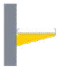
Load uniformly across the width of the cable tray
