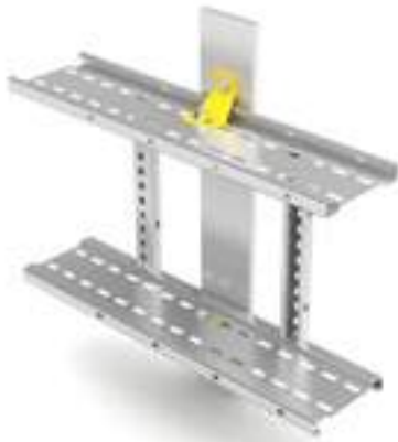
Safe working load 300kg per pair of adaptable fixing brackets when supporting edge mounted Speedway cable ladder
