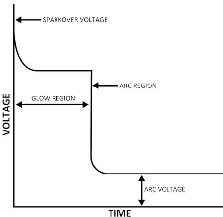
Typical operation characteristics of the Gas Discharge Tube (GDT) component used in the PDLVL100GP16.
