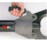
Hydraulic cutting head specifically designed to cut Copper and Aluminium cable having a max overall diameter of 95 mm.
