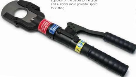
The blades are manufactured from high strength special Steel, heat treated to ensure a long service life. The head can be easily opened to allow the cutting of running cables. The head can rotate through 90 degrees, to enable the operator to work in the most comfortable position. HT-TC051 features an automatic safety valve to bypass oil when reaching maximum pressure; a pressure release device can also be operated at any stage of operation.
