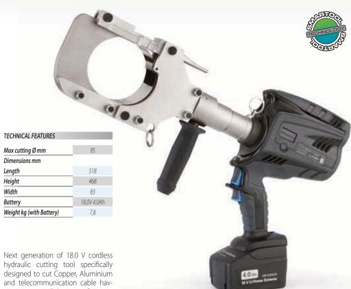
Next generation of 18.0 V cordless hydraulic cutting tool specifically designed to cut Copper, Aluminium and telecommunication cable having a max overall diameter of 95 mm. The blades are manufactured from high strength special Steel, heat treated to ensure a long service life. New Li-lon 18 V 4 Ah batteries offer a higher capacity than 14.4 V 3 Ah, while greater cutting speed and cutting force result from a revitalised hydraulic system with double speed action.
