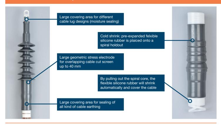
TC is a slim designed, uniform termination made of liquid silicone rubber used for indoor and outdoor applications. The terminations can be used as push-on or as cold shrink technique. The terminations are designed according to European Standard HD 629.1, IEC 60815 (sheet design shape), VDE 0278-629-1 and IEC 60502-4.
