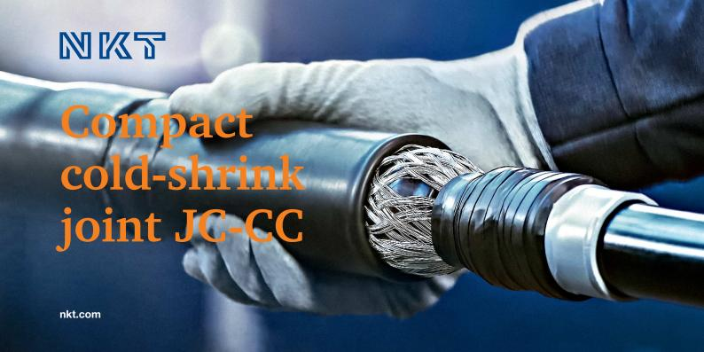
Our compact cold-shrink joint JC-CC for XLPE cables is state of the art. It uses flexible silicone rubber, which is placed onto a spiral and comes with pre-assembled components. During installation, the spiral core just needs to be pulled out and the flexible silicone rubber will then shrink automatically, thus making the installation easy, fast and safe.
